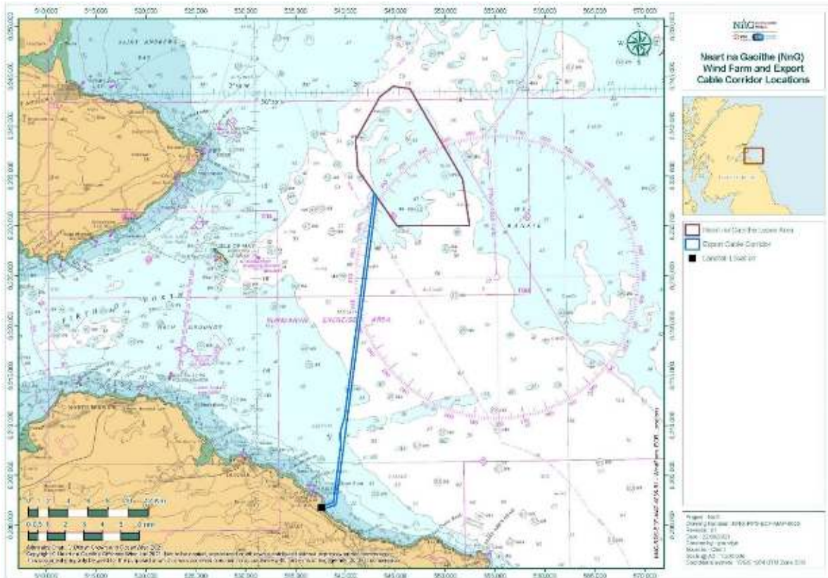
Figure 1 - Wind Farm Area and Export Cable
