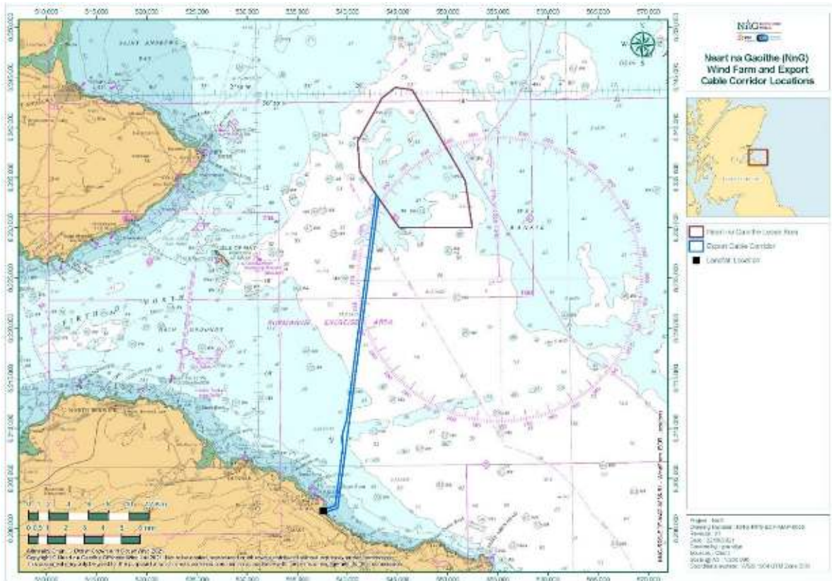
Figure 1 - Wind Farm Area and Export Cable
