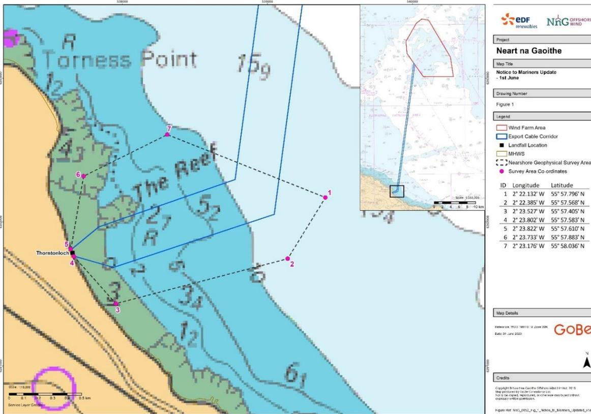
Figure 3 Area of nearshore boulder clearance operations
