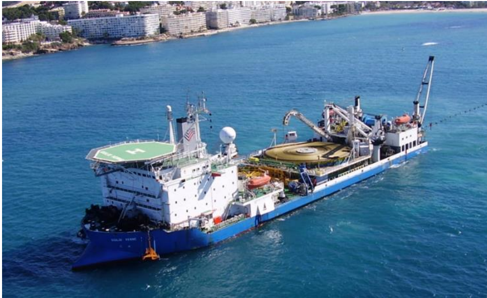
Illustration 4.18: Cable lay vessel Giulio Verne (Source: Prysmian Group)
