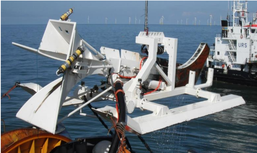
Illustration 4.16: Cable plough (Source: Prysmian Group)
